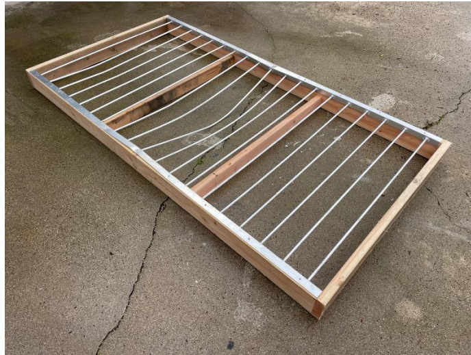
Photo No. 1 Test Specimen #1 after 4' (800 lb – ft) drop height
