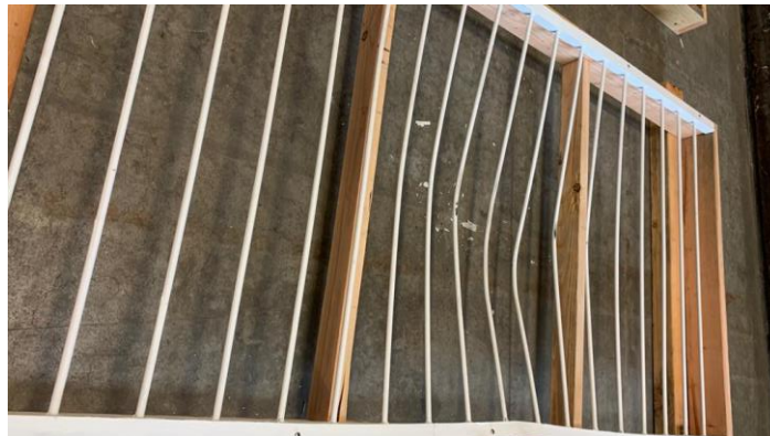
Photo No. 2 Test Specimen #2 after 4' (800 lb – ft) drop height
